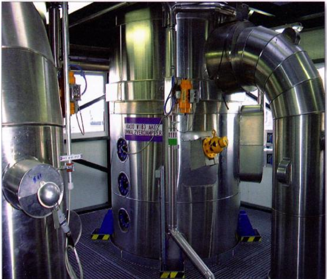
Melting crystallizer designed as evaporation crystallizer/熔融结晶器
