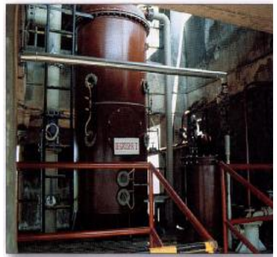
2-stages degassing plant in Indonesia/印尼一家二级脱气装置
