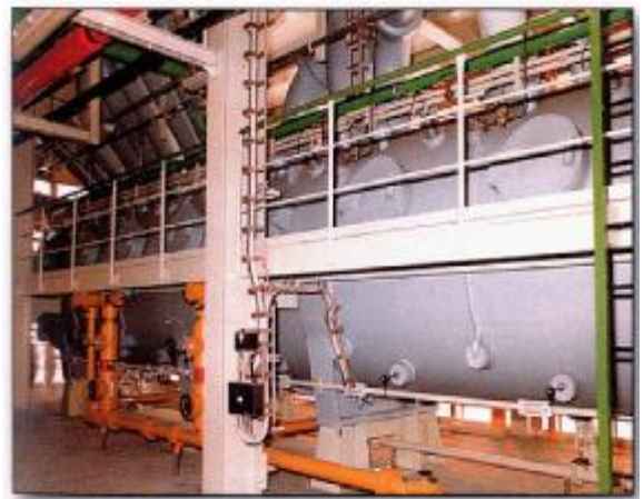
8-stage cooling crystallization plant/8 段结晶
